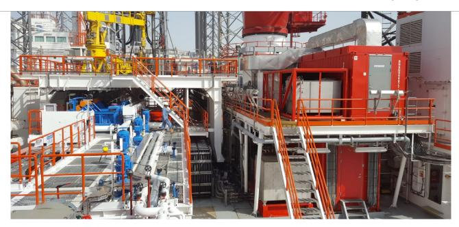
The Hytech Main Drilling Power System is a closed loop hydraulic power system (HPU). The flow and pressure control on the main pumps is very quick and accurate, which allows efficient and precise operation of the equipment. An extensive monitoring system ensures safety and gives the operator an overview of the system status. Typical applications are moving or rotary systems like hydraulic hoisting systems or Top Drive systems for the oil and gas industry.
